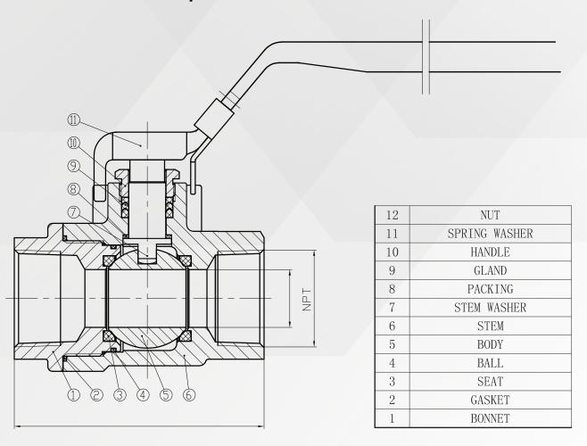
Refer to the diagram and parts list above for a detailed view of each component, assisting with installation, operation, and maintenance for optimal valve performance.
